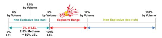
While noting the above, the assumption should be that a flammable atmosphere can be present at any time when working in a facility or tank vessel. It is therefore vital that all ignition sources are avoided.
