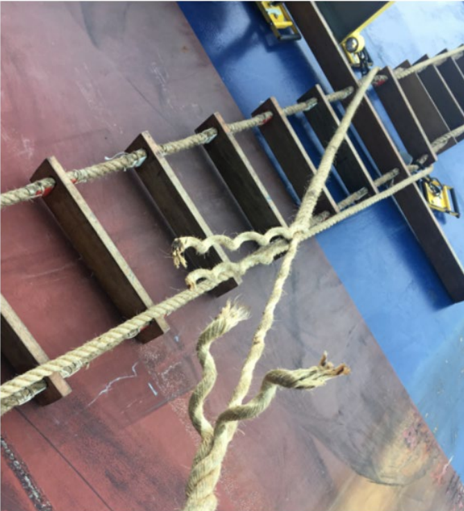
Example of an unsafe man rope
